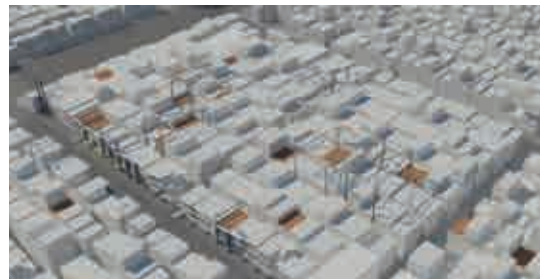
Structural pipes and service pipes superimposed on the existing to reinforce and allow for vertical expansion while connecting to infrastructure
