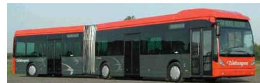
BRTS in Mumbai needs conventional buses with doors on right side also, similarly articulated and bi-articulated buses to achieve required capacities on the BRTS Network. Low floor buses are not a must as level boarding and alighting has been achieved very successfully in Ahmedabad Janmarg BRT as also in several other places in the world.
